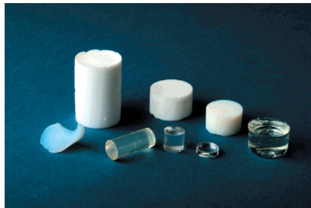
Figure 3. Monolithic, bridged polysilsesquioxane aerogels (blue-tinted or white) and xerogels (transparent).
